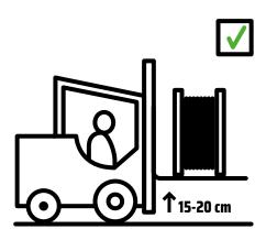
Insufficient lifting height may cause the drum to be dragged on the ground and eventually get damaged or dropped off the forks, especially if the ground surface is uneven. The drums may be placed and stacked on pallets to make it safer and easier to move them.
