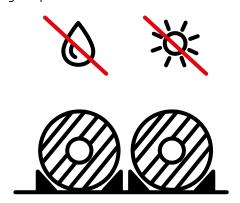
Cables with coloured outer sheaths shall not be stored in direct sunlight to prevent fading. Cables shall be protected against direct sunlight with suitable protective packaging, such as plastic sheeting.
