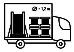
During transportation, the drum shall be fastened with a combination of wedges and transportation straps to tie down the front and rear of the drum, to prevent movement of drums.
