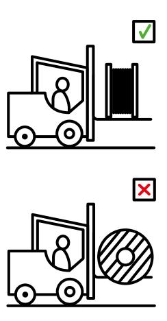
Lifting cable drums with a forklift is only allowed from the "flange side". To avoid damage, never touch the cable or its protective cover with the fork.
